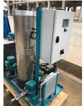
The varnish removal unit utilized by Saudi Aramco. Courtesy: CJC
