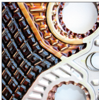
Varnish on plate heat exchanger
