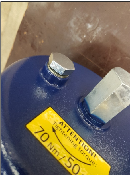
Figure 5: BEFORE - Location on the HDU15/25 for the CMU outlet hose connection. The air vent screw is reused.
