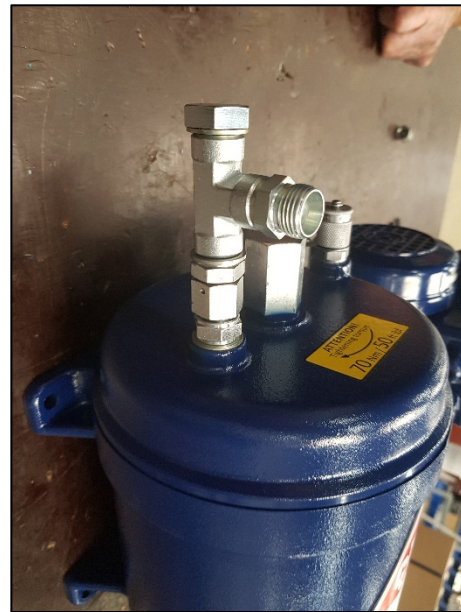
Figure 4: AFTER - Example of inserting a T-connection on the filter vents screw position to mount the hydraulic hose for the CMU outlet.
