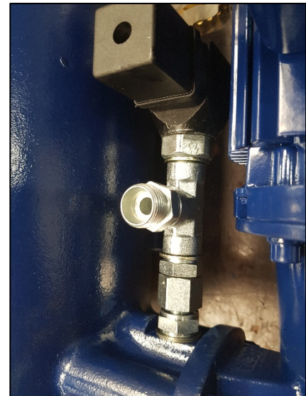
Figure 3: AFTER - Example of inserting a T-connection on the pressure side of the filter pump to mount the hydraulic hose for the CMU inlet
